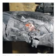
Major cable damage caused by thread contact
