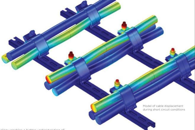
This technology enables a better understanding of the forces acting on various trefoil cable cleat designs, the stresses and deformations observed and the subtle changes in cable cleat design or materials which result in dramatic changes in performance.
