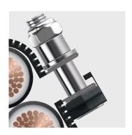
CMP Products' cable cleats use a partially threaded bolt in conjunction with the nut spacer, never allowing the cables to be exposed to the thread of the bolt. The use of these, along with cable cleat liners as standard, means the cables can only ever come into contact with smooth or flat surfaces.
