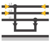
Fig 3. Phase-phase-to-earth short circuit
