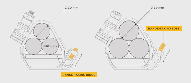
The Conqueror cable cleats are metallic cable cleats designed, constructed, and tested in accordance with the International Standard 'cable cleats for Electrical Installations' IEC 61914. The Conqueror cable cleat has been designed to restrain a large cable range take, and tested for exceptionally high short circuit conditions on cables held in trefoil application / formation, to ensure the securing and retention of cables without damage.
